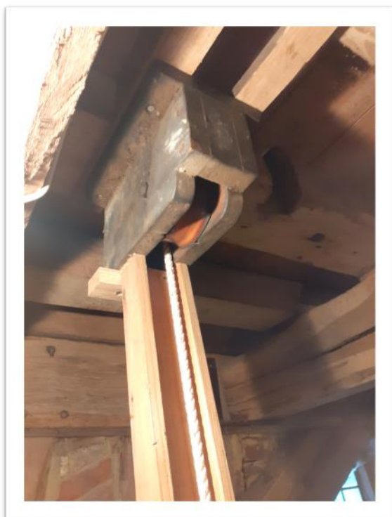
Repurposed old wooden pulley on the ceiling of the clock room to eliminate rope friction.
