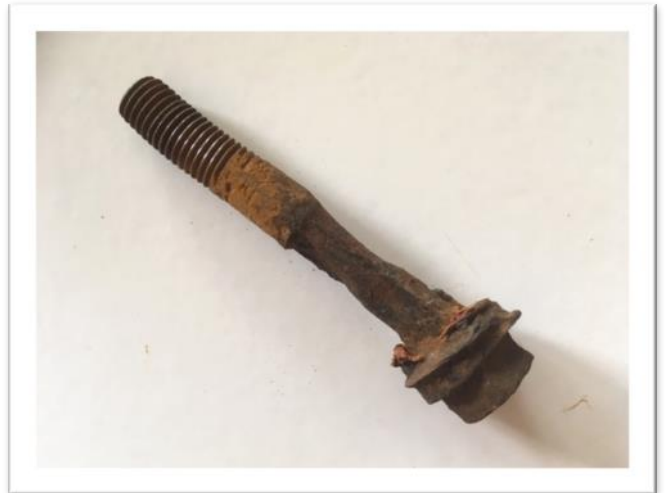
An example of a rusted headstock bolt
